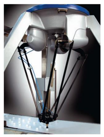
Precision is key! Motor feedback systems ensure precise positioning in packaging robots.
